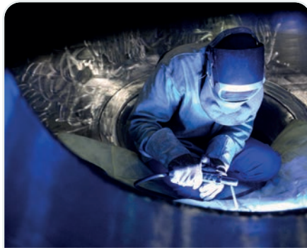
↑ Framatome, welding on an EPR steam generator ©Nicolas De Lepierre/Framatome
